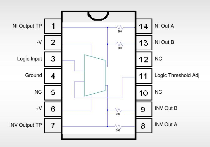
Unit provides two complementary outputs, and each output has a low-impedance output (no internal current limiting) which swings nearly from rail to rail, as well as two resistively limited outputs.
